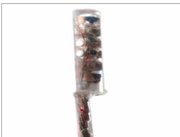
Figure 2. Microsensor, 8 mm long and 1 mm in diameter
