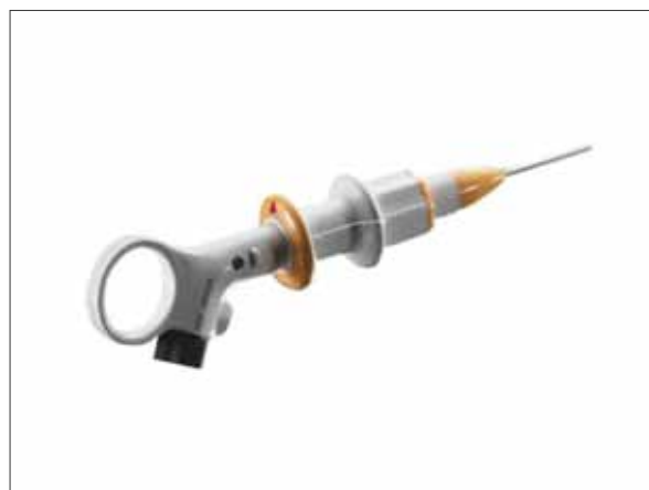
Figure 3. Proximal end of the Locatable Guide. Computer wire is connected at the black socket. Red arrow on the rotating knob is positioned in the direction indicated by the navigation system and the handle is squeezed to change the direction of the micro-sensor
